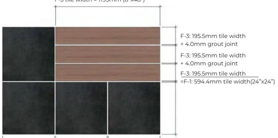
F-1 and F-3 tiles can be installed on-grid on Y-Axis with a grout joint of 1/8"
