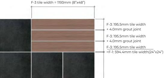
F-1 and F-3 tiles can be installed on-grid on Y-Axis with a grout joint of 1/8"
