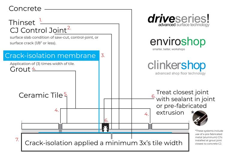
Crack Isolation (partial coverage): Apply an appropriate coat of Fracture Ban SC by Laticrete. 7. The crack suppression must be applied at a minimum of 3 times the width of the tile or stone being installed. Follow TCNA Method F125 for the treatment of hairline cracks, shrinkage cracks, and saw cut or control joints (see above).
